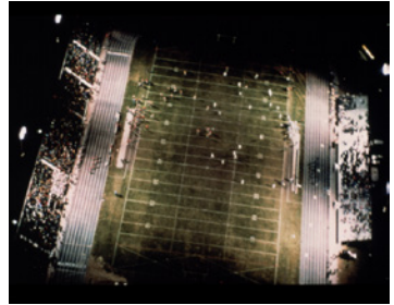
Misalignment of as little as 10 degrees shifts light off the playing field into the stands.
